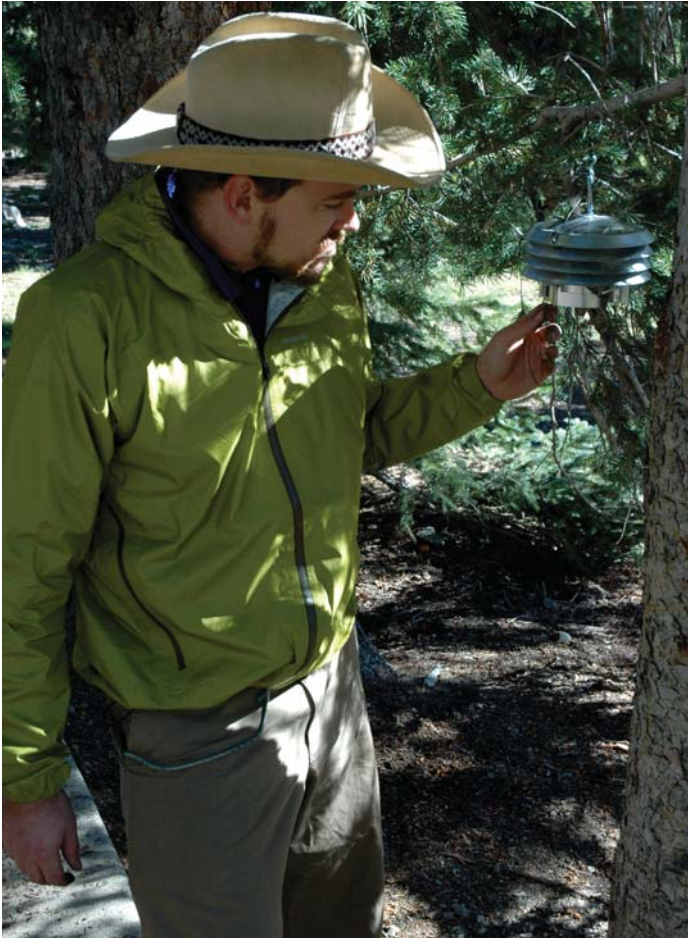
Figure 2. Jason Box installs a Lascar air temperature sensor.
